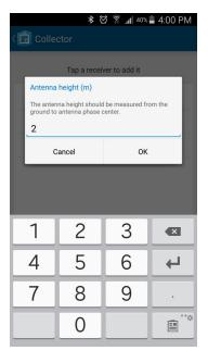
**Note:** If the elevation is irrelevant for your job, you can leave this blank. If you are doing RTK data collection, and your application requires elevation measurements, then enter an antenna height, taking into account the pole height, the antenna mounting plate and the antenna phase center offset.
