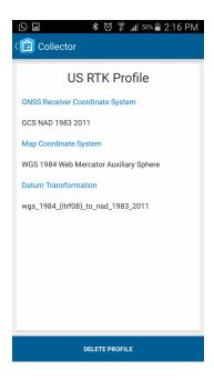
**Note:** If you are connected to an RTK network, the position output by the Arrow to collector will be in the same datum as the RTK network (for example: NAD 83 2011 usually in the US). Therefore it is important that you ask your RTK network provider for the datum information before creating your profile.
